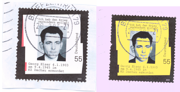
Fig. 1: Stamp used by the German Mail Office observed under natural light (left) and under UV light (right); while the paper background turns lightly violet due to the FWA present, the stamp turns to a vivid yellow as result of excited fluorescence. The UV content in natural light is not sufficiently high to excite the fluorescent pigment to detectable levels providing an easy way to prevent forgery.
